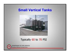
Relief valves set for 175 PSI, much lower than propane tanks which operate between 250 and 375 psi.
