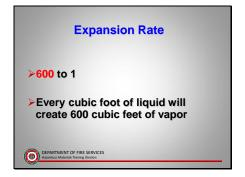
This is why Natural Gas is liquefied. For every truck load of liquid you would need 600 truckloads of vapor.
