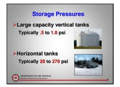
Relief valves for large capacity vertical tanks are usually set for ¾ of a pound. Large capacity vertical tanks hold millions of gallons of product. Horizontal tanks hold thousands of gallons.
