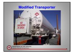
Storage tank has integrated UV, IR and CGI sensors with automatic shut-offs and alarms.
