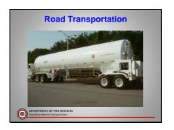
There are 3 distinct features of the LNG transporter. The size of the tank, the "bucket box" at the rear, and the pressure building coils under the belly of the tank. They are placarded 1972 and stenciled "Methane refrigerated liquid." This means that they are "dedicated" transporters and will only carry LNG.
